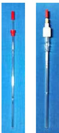
Standard (left) and air sensitive (right) photoNMR tube assemblies.
