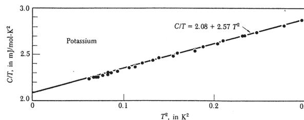
FIG. 1: Experimental values of heat capacity for solid potassium. The figure copied from the book [1].
